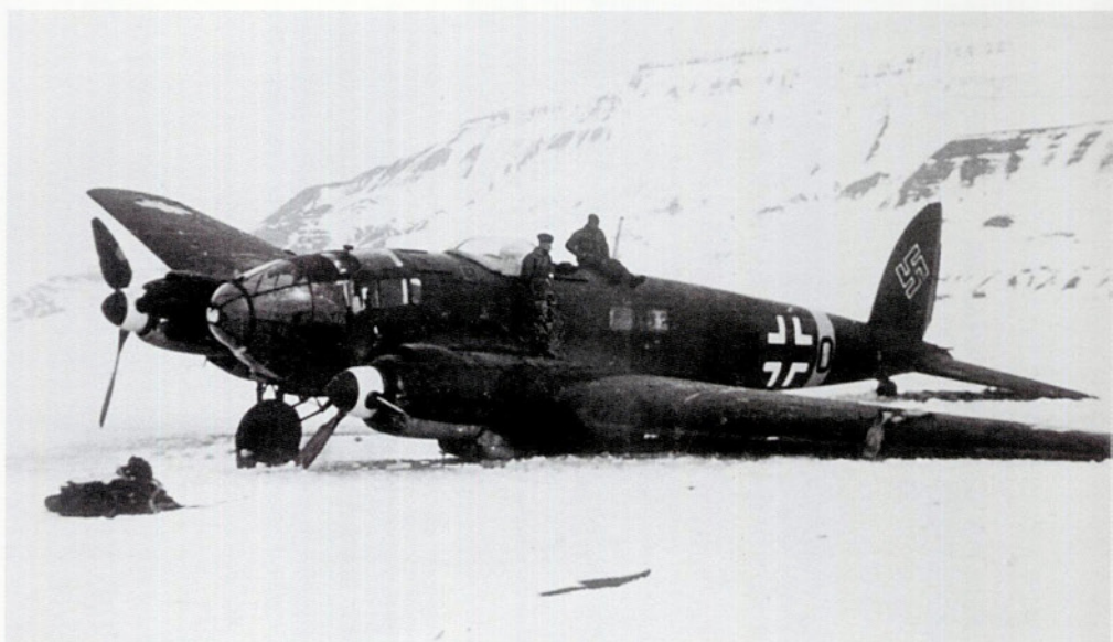
RIGHT: In the harsh freezing conditions that prevailed in northern Norway and Finland, take-off and landing accidents occurred frequently. The port undercarriage leg of this He 111 apparently collapsed just as the aircraft completed its landing run.
