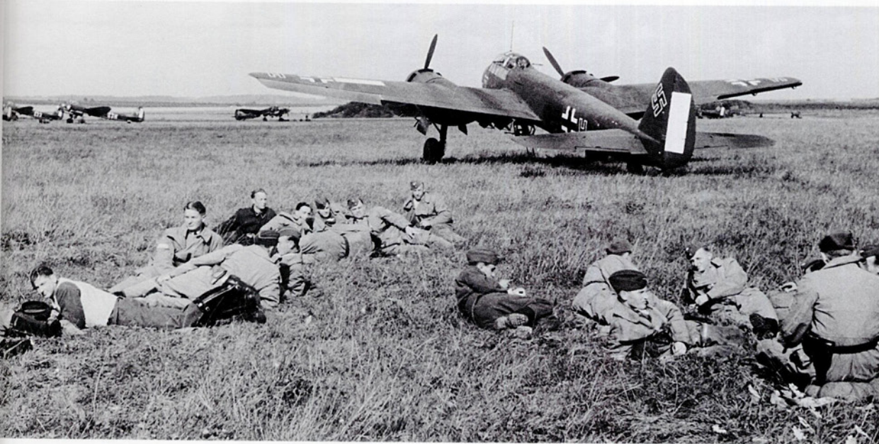
LEFT: During the Battle of Britain many Luftwaffe bomber aircraft had white vertical bars painted on top of their wings and on their rudder to easily identify their Gruppe when operating in close formation. These Ju 88 A-1s from I./KG 77 carried a single such bar in each position.
