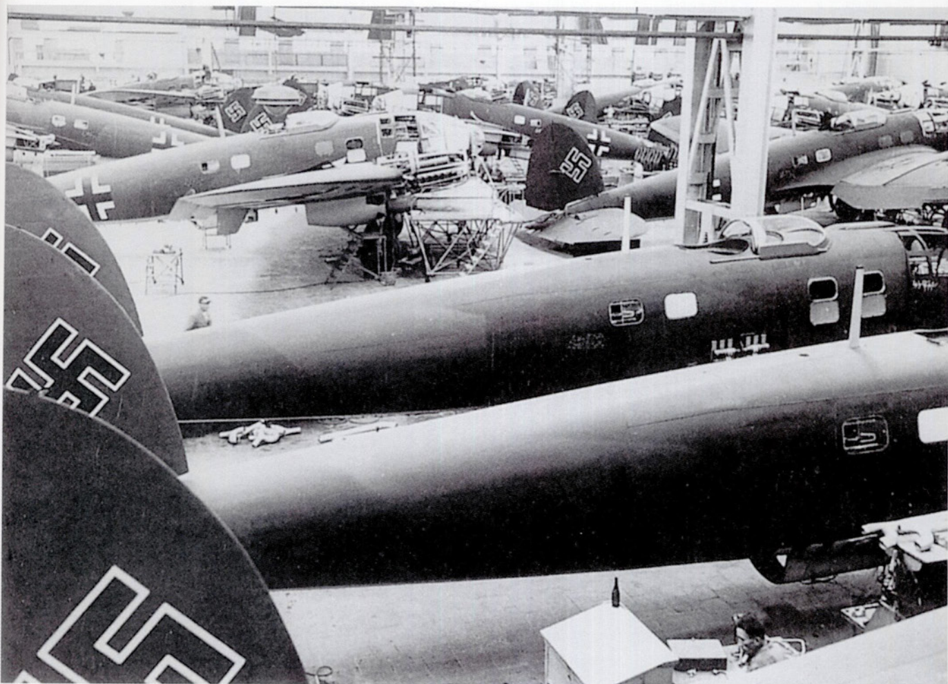
ABOVE AND RIGHT: Two more photographs of He 111 H-6 fuselages under construction, this time before the national insignia have been applied. All He 111s built at the Oranienburg factory during the first half of the war had their Stammkennzeichen four letter call signs painted white.
