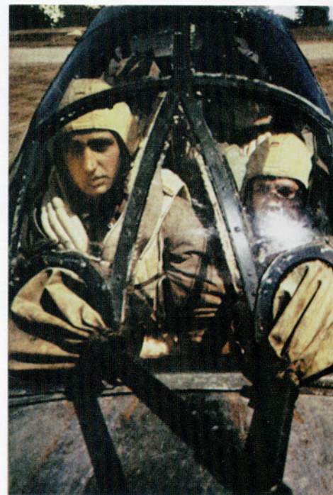
BELOW: This photograph shows graphically the cramped conditions for the crew of the Ju 88 when attempting to operate the two rearward firing 7.9 mm MG 17 machine-guns simultaneously.
