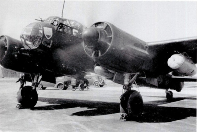
BELOW: This photograph shows a Ju 88 A-4 with Walter 109-500 rocket engines mounted beneath each wing belonging to 1./KGr 506, S4+AH, and carries the unit's badge described opposite.
