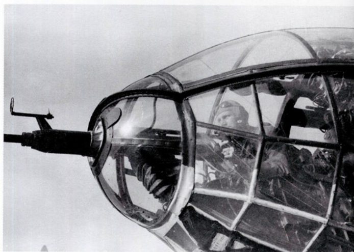
BELOW: This close-up of the nose of an He 111 H-10 clearly shows the hand-held 20 mm MG FF cannon and the ridged lines of the balloon cable cutting device which formed part of the canopy frame. Early experiments with a special outrigger structure for cutting balloon cables proved too cumbersome and the device was replaced by that seen here
