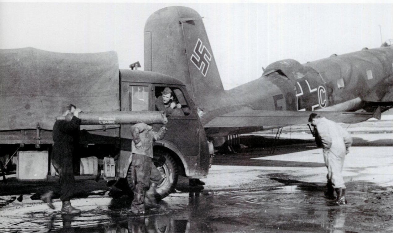
LEFT: Two mechanics carry a cylinder, used to top up the on-board oxygen supply, towards a Focke-Wulf 200 of 7./KG 40. This Condor carries the standard camouflage pattern of RLM 72 and 73 with the code F8+CR in black and the individual letter 'C' edged in white. On many Fw 200s the fuselage Balkenkreuz had narrow white outlines.
