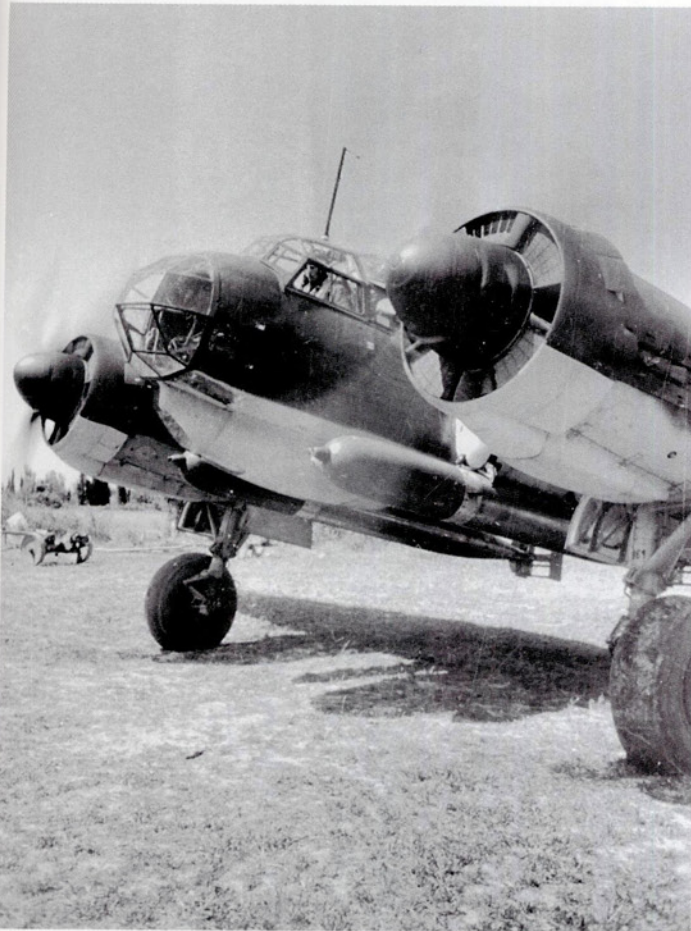
ABOVE: Late in 1941 Luftwaffe anti-shipping aircraft gained a new weapon when the air-launched torpedo was introduced into service. This Ju 88 carries two such weapons under the wing centre section.
